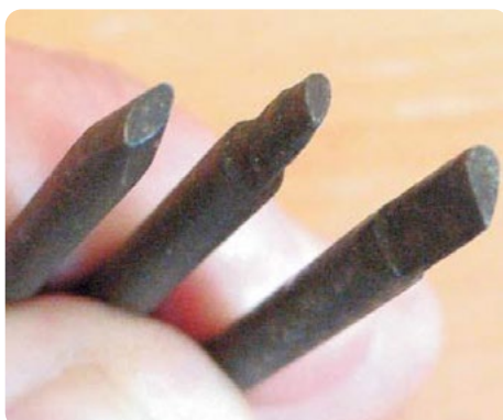
Photo 11. Homemade punches make it easier to clean up the small recesses of the eyelets
