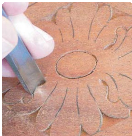
Photo 9. Cutting out the four eyelets in the design using tool #3
