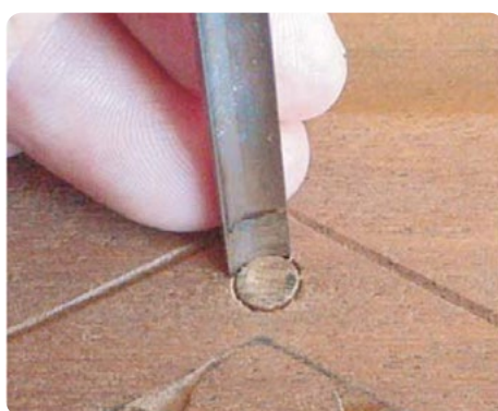
Photo 12. Setting in the four circles in the border with tool #2
