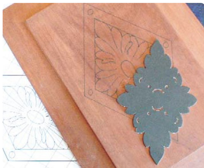
Photo 5. A stiff card template makes it easier to transfer the design to the wood
