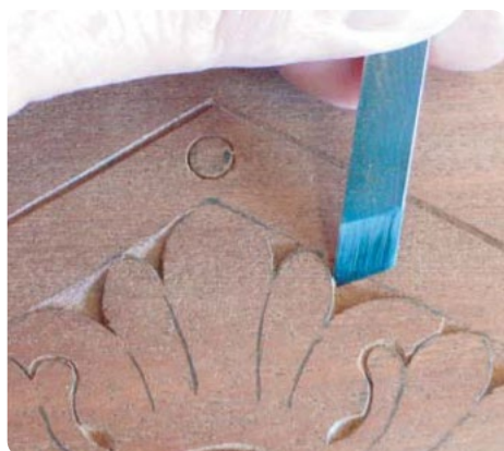
Photo 8. Defining the leaf design from the border using chamfers
