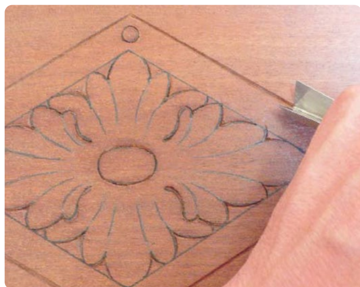
Photo 6. Setting in the V-line around the diamond shape
