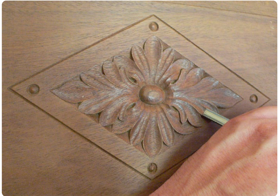
Photo 19. Carving the final leaves, removing all flat areas from the acanthus carving
